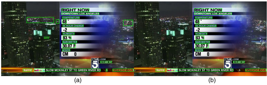
Fig. 13 a is an exemplary text detection result of standalone analytical method, b is the result after the machine learning verification. Some repeating patterns such as e.g., windows, tiles, and light sources from the analytical detection result have been removed by machine learning verifier
